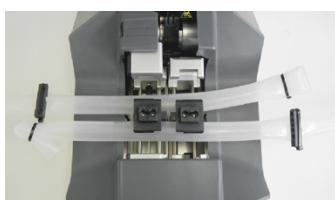
3. Insert the tubes into the tube holder and close cover.
