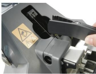
The welding is finished when the cover opens.
