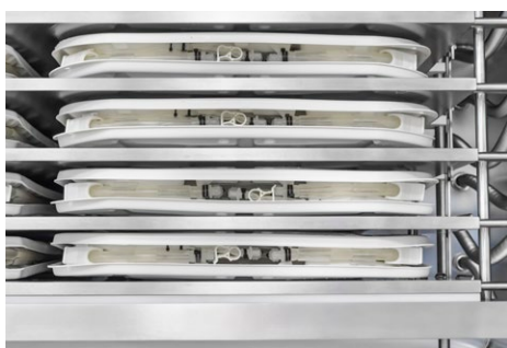
Celsius® FFTp containers between plates in the freezer
