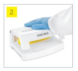
Apply slight uniform pressure with your hand to start sample clarification. You will feel a certain resistance while liquid is pressed through each membrane.
