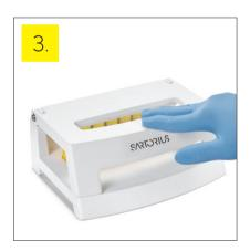
Press down on the station lid so that the left and right corners touch the base plate. Hold the lid in place for 3 seconds to ensure all sample liquid is filtered through.
