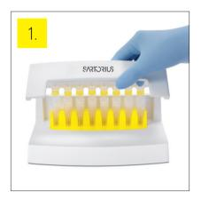
Close the station lid. The grooves align the caps automatically, securely sealing every single Claristep® Filter unit for the most convenient processing.
