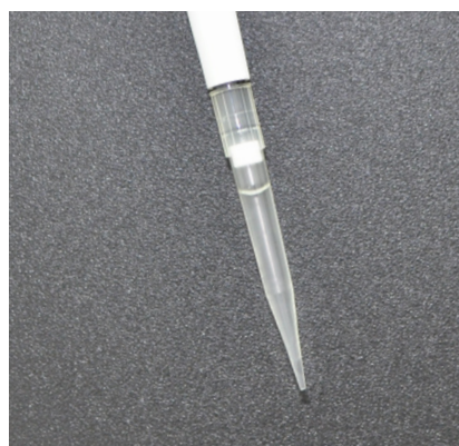
Figure 2. Pipetting BSA solution (1 mg/ml) with slow speed (Picus® 2 setting 1) is gentler on the protein.
