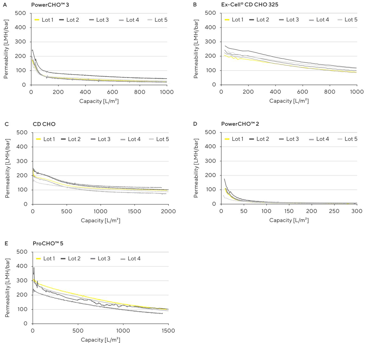
**Figure 2:** Permeability Versus Capacity. Consistent Lot-To-Lot Filterability Performance for 5 Different Cell Culture Media Tested With 4 - 5 Different Membrane Lots of Virosart® Media Filter Each at 2.0 bar | 30 psi.
