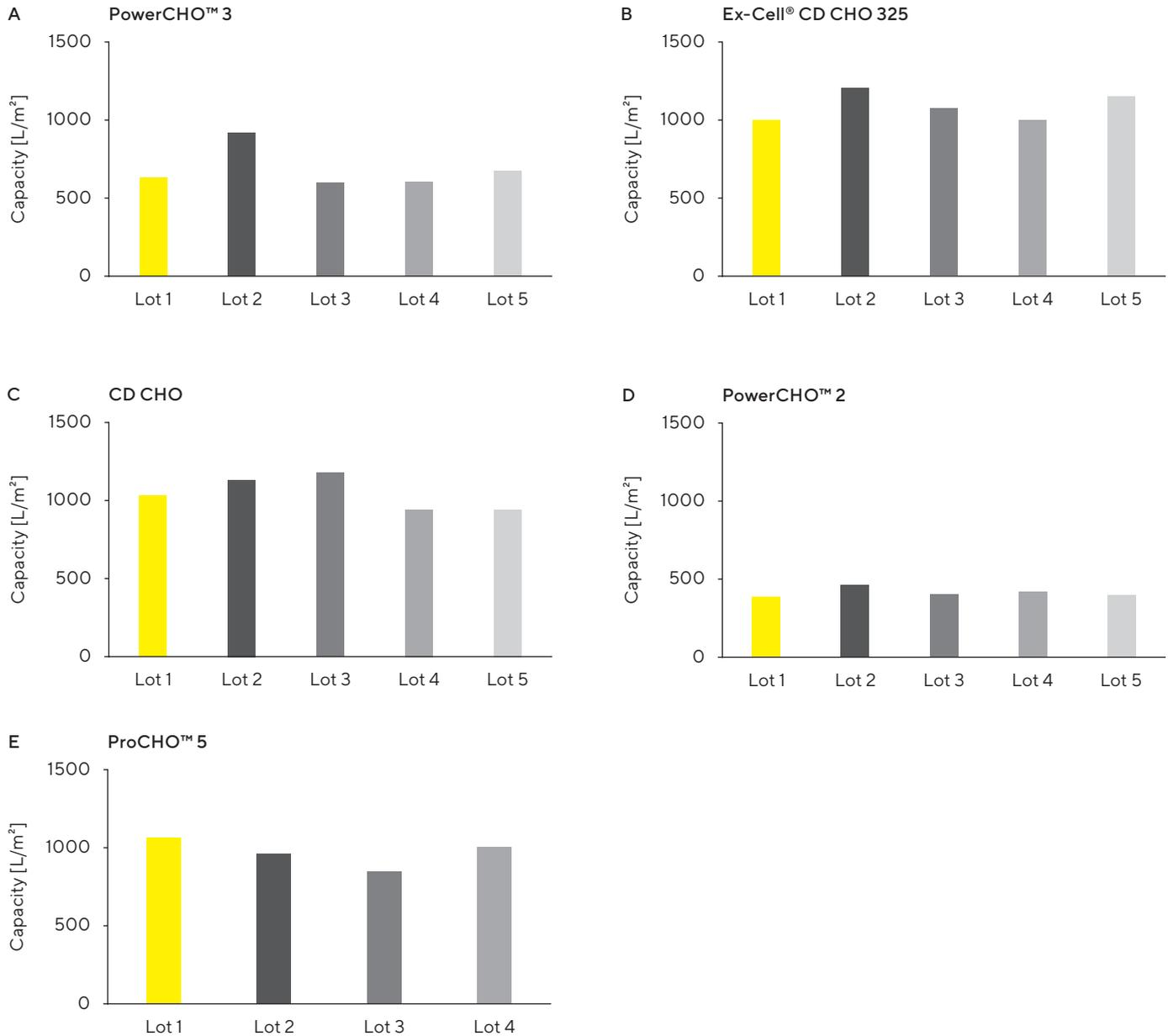
**Figure 3:** Lot-To-Lot Filter Performance Consistency [L/m<sup>2</sup>] Tested With 4 to 5 Different Membrane Lots of Virosart® Media Filter for 5 Different Cell Culture Media After 4 Hours of Filtration at 2.0 bar | 30 psi.
