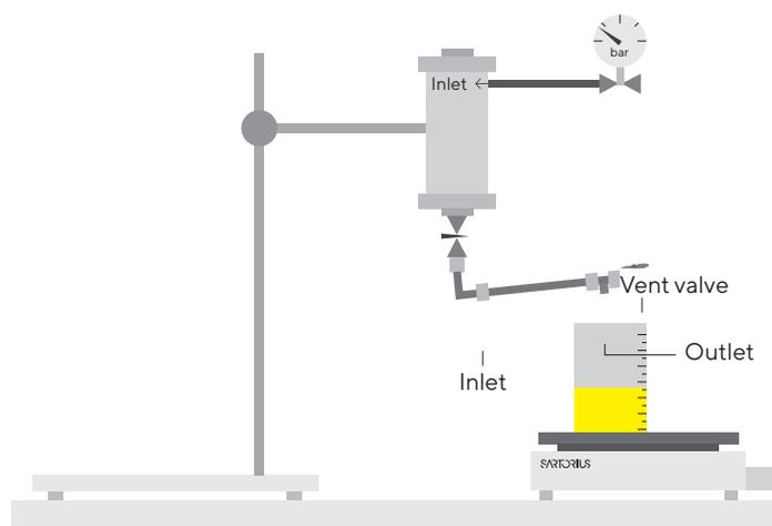
**Figure 1:** Experimental Set-up of Small-Scale Filtration Using Virosart® Media Lab Modules
