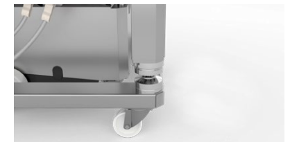
Weight control (Picture of one load cell)
