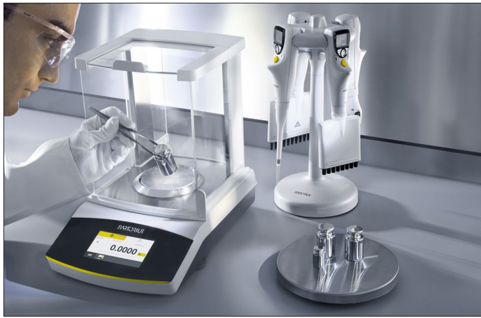
Figure 3: Checking the accuracy of laboratory balances with external test weights.
