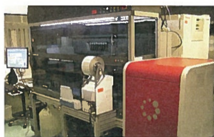
Picture: The Octet 384RED integrated to a Tecan Freedom Evo workstation via a docking station. The operation of the Octet 384RED is controlled by the Tecan EVOware software. The Tecan integration enables inter alia the tray-wise (96 biosensors simultaneously) off-line regeneration of Protein A biosensors and the off-line coating of Amine Reactive biosensors using the Tecan TE-shake platform, thus streamlining label-free analysis.
