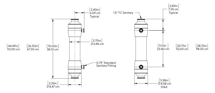
Bioproducer Exact length for different Fiber length: 12, 24 or 41 inch
