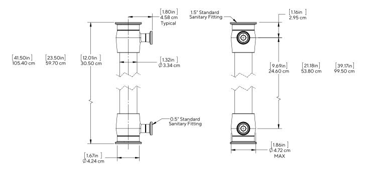
Mini Bioproducer Exact length for different Fiber length: 12, 24 or 41 inch
