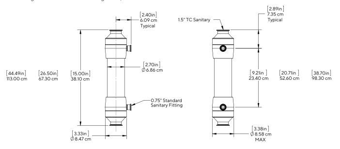
Bioproducer Exact length for different Fiber length: 12, 24 or 41 inch
