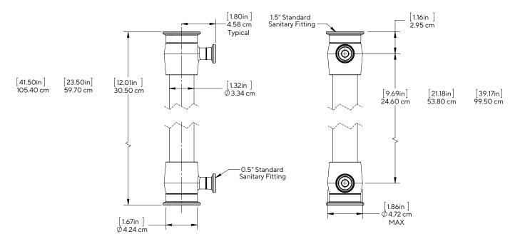
Mini Bioproducer Exact length for different Fiber length: 12, 24 or 41 inch
