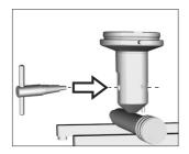
Insert the valve stopcock into the manifold until the rear stop. The handle's thinner, shorter side must point toward the left.
