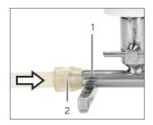
Fix the manifold (1) with one hand and use the other hand to connect the quick coupling (2) with the hose to the manifold plug-in nipple.
