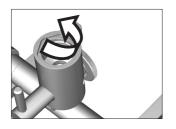
Carefully remove the O-ring from the groove.
