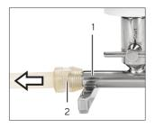
Hold the manifold (1) with one hand and use the other hand to pull the hose with the quick coupling (2) from the manifold connector.
