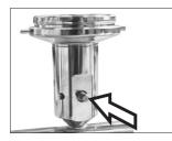
Fit the valve stopcock with your left hand, and use your right hand to install the knurled screw with spring in such a way that the spring is vertical, or that the spring is in the groove of the manifold.
