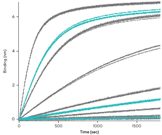
Note. The Octet® Sample Diluent was used as the matrix and all samples were analyzed in quadruplicate (binding curves corresponding to Standard Samples (gray) and Spiked Samples (teal)).
