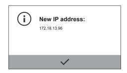
If the IP address of the scale changes, e.g. after the DHCP server allocates a new address, an info message notifies the user of the change.
