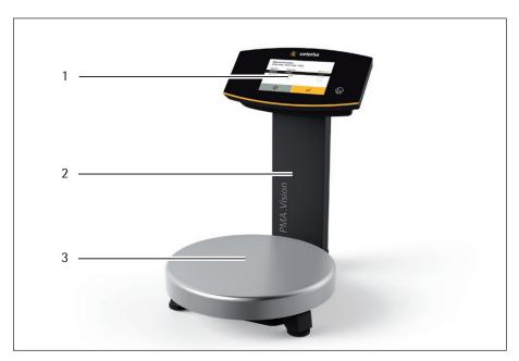
Fig. 1: Scale front view
