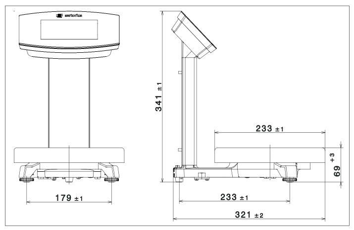
Fig. 1: Device dimensions PMA.Vision VIS1X (information in mm)
