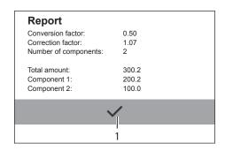
According to the display, 300 o was poured in, but the container actually contains 150 g by weight in accordance with the factor you selected.
