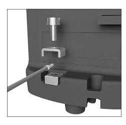
► Connect the cable lug of the equipotential bonding cable to the grounding terminal of the scale.
