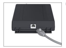
Connect the link cable to the ex-link converter.
