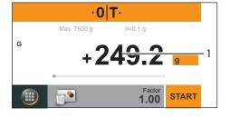
You can read the measured value as soon as the weight value (1) stops changing and the unit is displayed.
