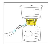
1. Unpack the filtration unit (Sartolab® RF|BT). If using a filtration unit without a bottle (Sartolab® BT), screw the funnel onto a bottle with a 45 mm thread. Connect the vacuum connection of the Sartolab® RFIBT unit to a vacuum source. If necessary, use the tube connector. See also the Instructions for Use supplied with the Sartolab® RF|BT units for more detailed information on the filtration. process.
