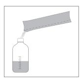
2. Use the appropriate number of filter aid pouches per filtration unit (see Chapter 6 'Typical Performance Specifications'). Open the pouch(es), pour the filter aid into the cell culture, and mix to homogenize. Discard the empty pouches.
