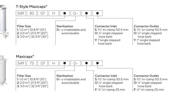
(Optional with vent valve design for connection of integrity tester. Example: 5497307H1G-SOIT)
