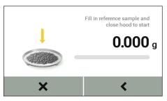
▶ Place the sample pan with the "ReproEasy pad" (accessory) reference sample on the pan support.
