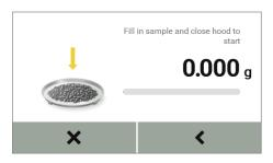
Place the sample on the sample pan or filter(s).
