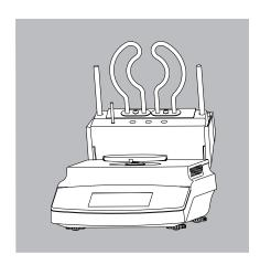
3) Clean the heating element and temperature sensor with a weak solvent such as ethanol.
