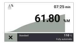
If no target value is set, the measurement process is displayed as a curve diagram.
