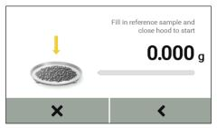
▶ Place the sample pan with the "ReproEasy pad" (accessory) reference sample on the pan support.
