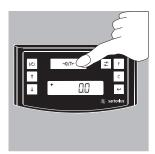
If a different value is displayed: Tare the scale using the [->0,TFE] key (Zero/Tare).
