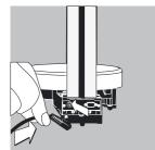
Insert the right-angle plug into the IEC jack (13) on the scale
