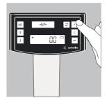
2. Press the F formulation key (7) several times to select the conversion factor ".25" used in this example.
