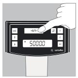
Center the calibration weight on the weighing pan (11). Calibration/adjustment is performed automatically.
