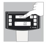
If a different readout is displayed, zero or tare the scale using the  $\boxed{\text{vore}}$  key (5).
