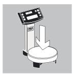
• Place the weighing pan on the scale.
