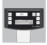
After the scale has been turned on, it will automatically run a self-test. At the end of this test, 0.0 g is displayed.
