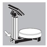
• Ground the scale. Connect the cable to the grounding terminal (14).
