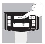
1. Place the empty paint can on the weighing pan and tare (zero the display).
