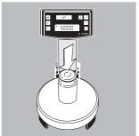
Center the calibration weight on the weighing pan (11).
