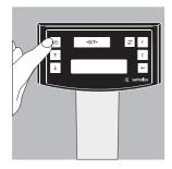
Turn on the scale using the key (2).
