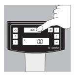
1. Place the empty paint can on the weighing pan and tare (zero the display).
