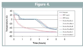
Freeze Profiles Shown to be Independent of Bag Placement. "HTF supply" and "HTF return" denotes the temperature of the heat transfer fluid when entering and exiting the freeze units. "ProductRearBayA" denotes the freeze profile for the bag placed in the front section of bay A. All other labels follow the same naming system.
