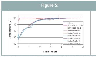
Thaw Profiles Shown to be Uniform and Reproducible. "HTF\_Outlet\_Temp" and "HTF\_Inlet\_Temp" denotes the temperature of the heat transfer fluid when entering and exiting the freeze units. "Setpoint shows the target setpoint of the heat transfer fluid. "ProductRearBayA" denotes the freeze profile for the bag placed in the front section of bay A. All other labels follow the same naming system.
