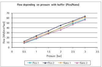
Flow rate  $>10 \text{ MV/(min} \times \text{bar)}$
