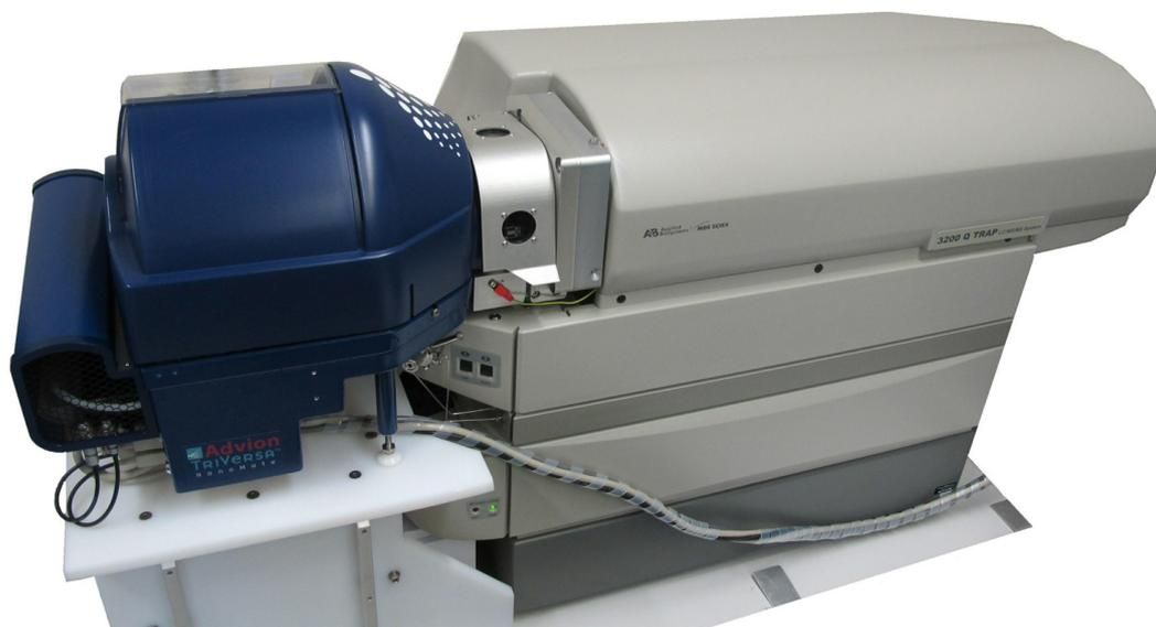
Note. An Applied Biosystems/SCIEX 3200 QTRAP featuring hybrid triple quadrupole/linear ion trap capabilities was used for the mass spectrometry analysis. NanoESI was ensured by the TriVersa NanoMate, a chip-based ion source. The Agilent HPLC system is not shown. (Image credits: Department for Plant Biochemistry, Albrecht-von-Haller-Institute for Plant Sciences, Georg-August University of Göttingen, Germany.)
