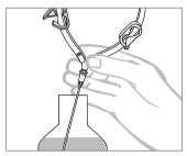
For filling with the 6-cm metal needle from an open culture broth container: remove the broth by pumping through the metal needle.
