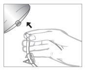
Insert the male luer connector of the adapter into the bag with the female luer luer lock fitting.
