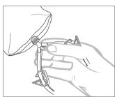
Switch on the pump to transfer equal volumes of the sample into the two Sterisart® NF containers; at the same time, the plastic bag deflates as the vacuum builds up inside.
