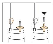
Tightly seal the two vent filters using the enclosed rubber caps.
