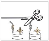
Seal off the two tubes just above the Sterisart® NF containers by closing the pre-installed tube clamps. Cut off the tubes above the clamps.
