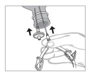
For filling with the 6-cm metal needle from a closed culture broth container: pierce the container closure with the metal needle and with the sterilizing vent filter spike.
