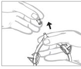
Attach the 6-cm metal needle supplied to the Y-distributor to remove washing solution from open containers.
