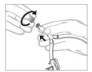
Turn the plug clockwise to detach it from the removable double luer lock adapter.
