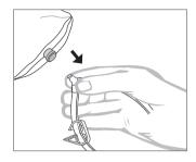
Attach the 6-cm metal needle supplied to the male luer connector on the Y-distributor to remove washing solution from the open containers.
