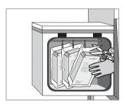
Open the box or, if appropriate, pass the closed Sterisart® NF boxes through the air-lock port on the isolator.
