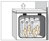
Sterilize the outer surface of the box according to the isolator validation specifications, for example, with  $H_2O_2$ .
