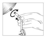
Turn the double female luer lock adapter (removable) on the Sterisart® NF system clockwise to connect it to the bag with a male luer lock fitting.
