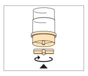
Switch off the pump. Tightly seal the outlet of each Sterisart® NF container with a plastic wing nut plug, twisting it about half a turn clockwise.
