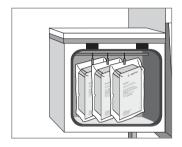
Place the individual packs, still enclosed in the gas-impermeable box, in the sterilization area.
