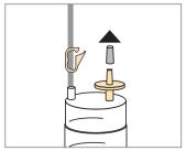
Remove the rubber caps from the vent filters.
