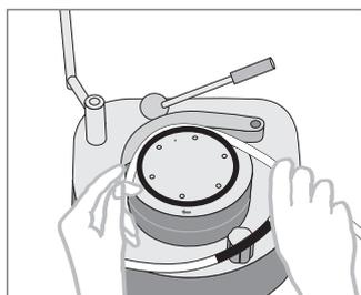
Thread the tube without the black rings (not color coded) in the pump head, following the instructions given for the pump used.
