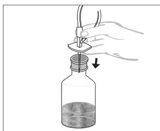
Insert the double-needle metal spike without color coding (the shorter of the two double-needle spikes) as far as necessary into the upright bottle filled with slightly soluble powder.
