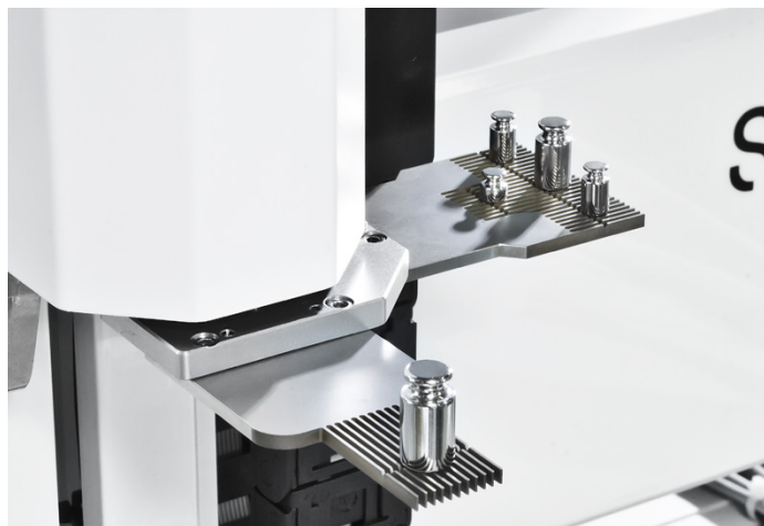
Picture 4: Dual arm system with multi-weight-and single weight handlers
