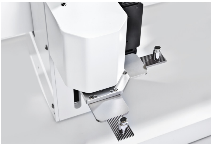
Picture 3: Dual arm system with two single weight handlers
