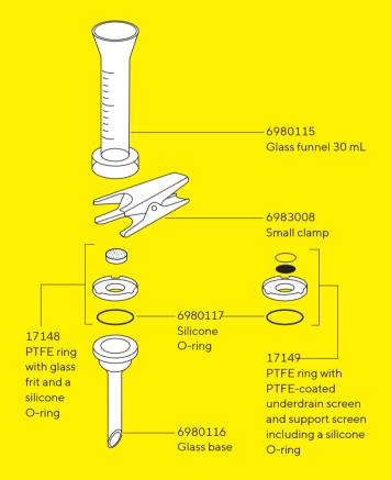
Note: PTFE rings in sets 17148 and 17149 have different dimensions and are not interchangeable.
