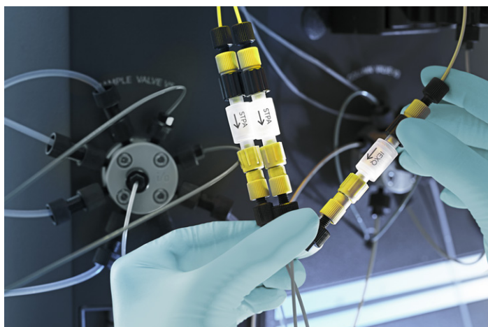
Fig. 1: Sartobind® Pico installed on a liquid chromatography system.
