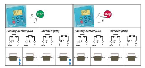
If **STOP** is pressed the remote stop/start switch will have no effect.
