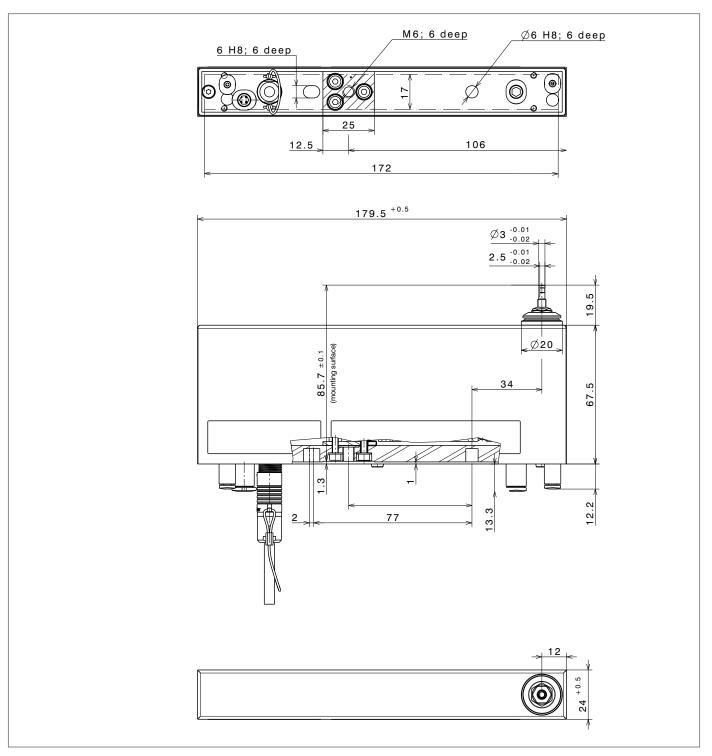
Fig. 12: Dimensions for model WZB25-NC (in mm)
