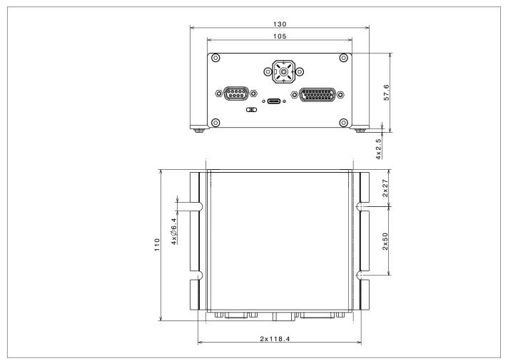
Fig. 15: Dimensions for electronics unit (mm)
