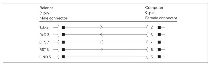
Fig. 9: Cable type: AWG 24 specification
