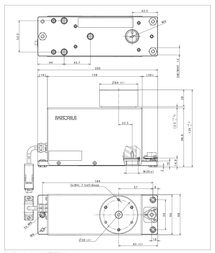
Fig. 11: Dimensions for model WZB8202-N (in mm)  $\,$
