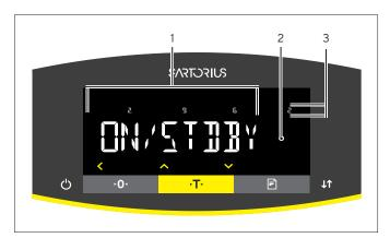
Fig. 8: Menu and system settings display (example)
