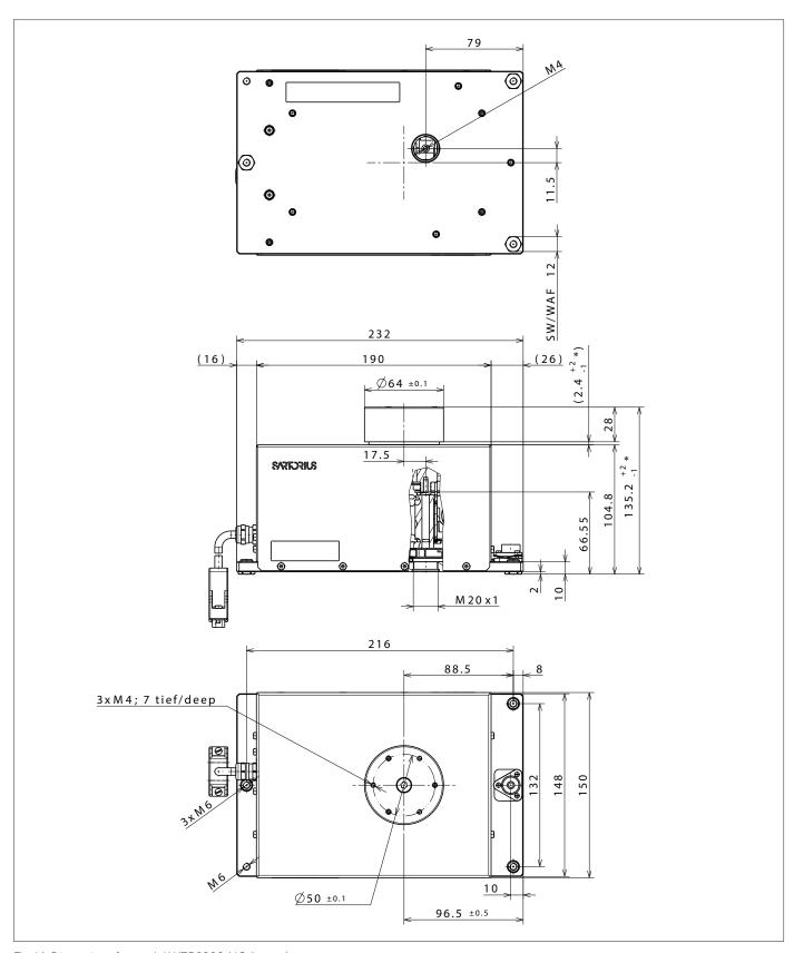
Fig. 14: Dimensions for model WZB8202-NC (in mm)  $\,$
