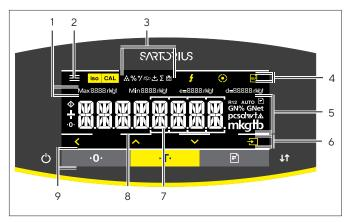
Fig. 7: Operating display in weighing mode (example)
