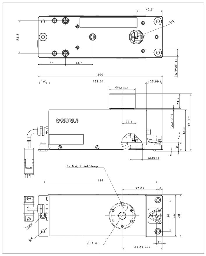
Fig. 10: Dimensions for models WZB254-N |-ND, WZB653-N and WZB1403-N (in mm)
