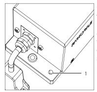
On the reverse of the weigh cell mounting plate, thread M6 (1) is available for a potential equalization conductor (e.g., for a spatula).
