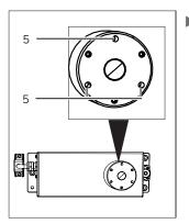
▶ If required: Screw the user-specific load holder onto the thread (5) of the load receptor (for torques, see Chapter "5.11 Maximum Load on the Pan Support", page 16).
