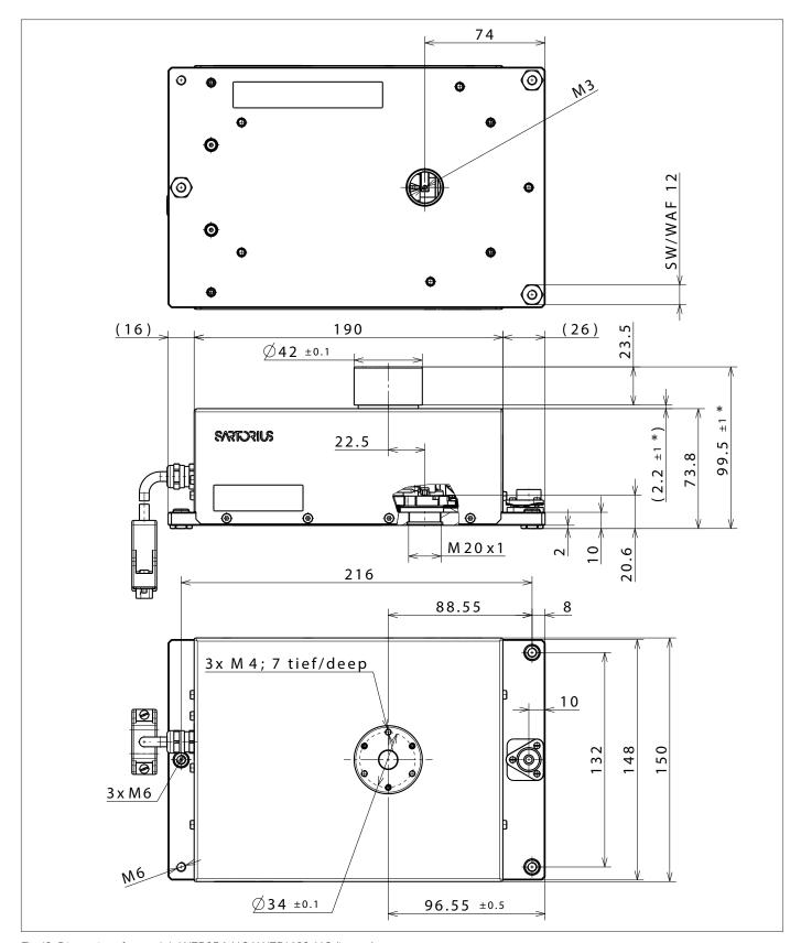
Fig. 13: Dimensions for models WZB254-NC | WZB1403-NC (in mm)  $\,$
