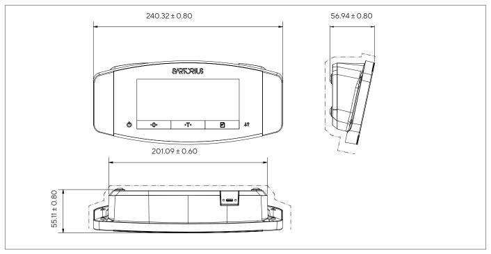
Fig. 16: Dimensions for optional YRD01 display unit (in mm)
