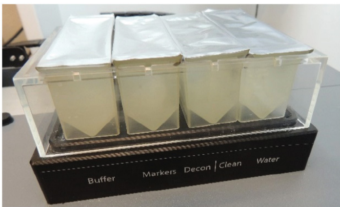
Figure 1: Fluid Station. Marker Cartridge should always be installed at the “Markers” location.
