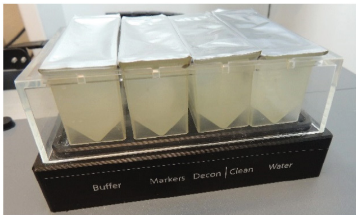
Figure 1: Buffer should always be installed at the first, left most position.
