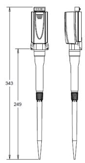
Figure 6. rLine models dimensions with tips
