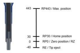
Figure 3. Base addresses and positions for rLine 50-1000ul LS
