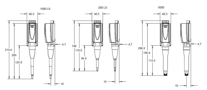
Figure 5. rLine models dimensions without tips
