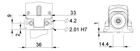
Figure 7. rLine location guide dimensions
